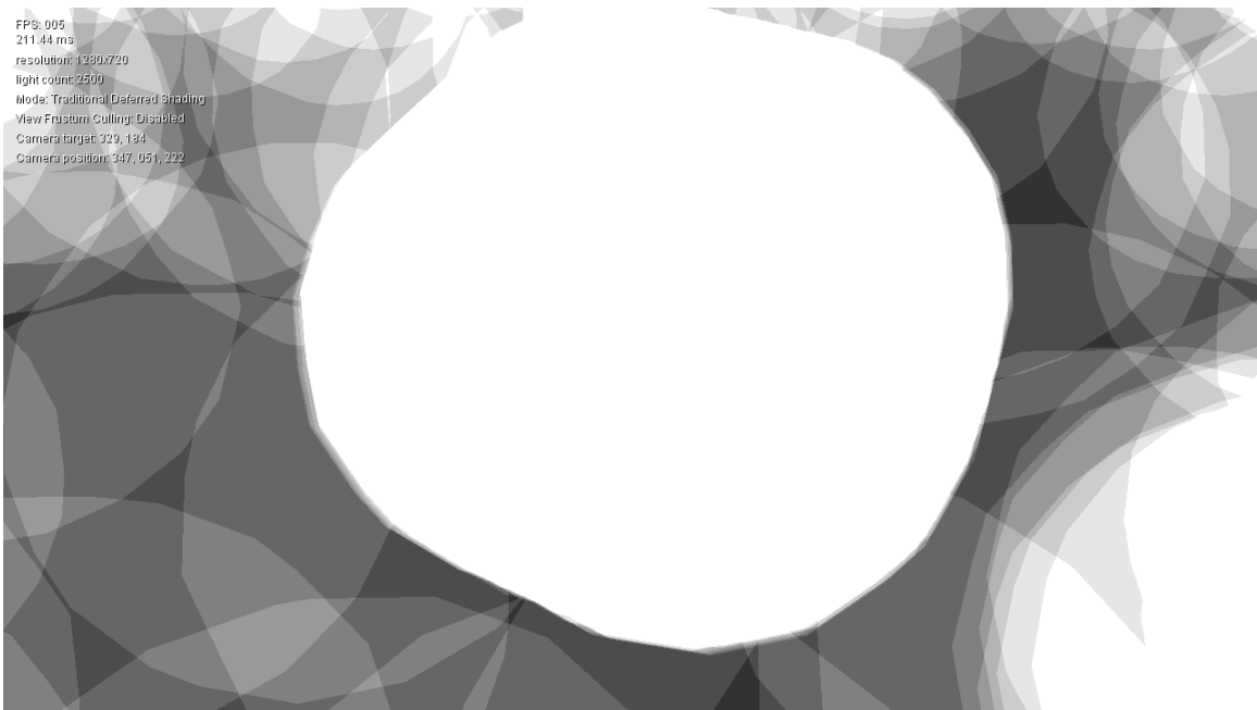
Number of lights for traditional Deferred Shading (white = more than 10 lights, black= 0 lights)
